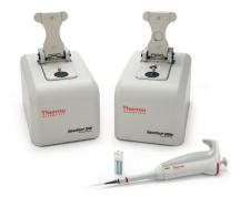
Using the patented NanoDrop microvolume sampling technology, a 1  $\mu L$  sample can be measured in less than 5 seconds. Simply pipette a 1  $\mu L$  sample directly onto the pedestal, measure and wipe clean. In addition to the pedestal, the NanoDrop 2000c instrument offers a cuvette position for larger volumes.
