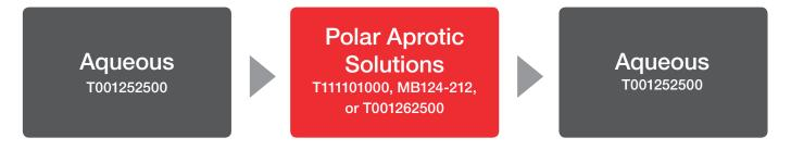
A thorough aqueous wash before and after using organic solvents can help to prevent the precipitation of proteins that can clog your instrument, cause sample contamination, and potentially cause premature replacement of your columns. Using the appropriate process will optimize peak shape, keep baselines smooth, and prevent precipitation.
