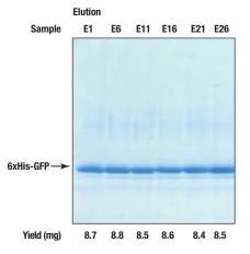
with 10 CV of MES buffered saline (20mM MES pH 5.0, 300mM NaCl) to remove imidazole, and then 10 CV of ultrapure water, followed by equilibration with 10 volumes of binding buffer containing 5mM imidazole. A lysate challenge was included every fifth cycle for a total of 20 blank runs and six lysate challenges (runs 1, 6, 11, 16, 21 and 26). 6xHis-GFP yield and purity were similar for all lysate challenges as seen by protein estimation with the Pierce 660nm Protein Assay and SDS-PAGE.
