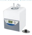
Ideal for sterilising small research tools including forceps, scissors, scalpels etc. Eliminates the danger of open flames by heating included glass beads to 300°C, eliminating bacteria, spores and other microorganisms.
