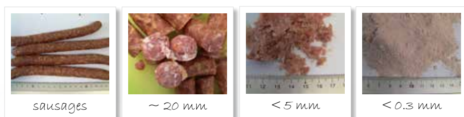
Figure 3: Homogenization of sausages; from left to right: original sample; pre-cut with large fatty parts; ground to < 5 mm; pulverized sample < 300 µm
