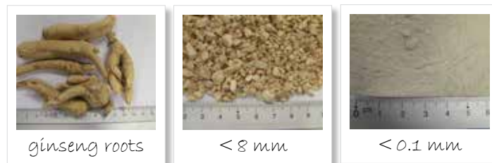
Figure 8: Homogenization of ginseng; left to right: original sample, sample ground to < 8\text{ mm} , sample ground to < 100\ \mu\text{m}
