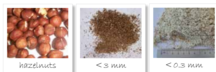
Figure 5: Homogenization of nuts; from left to right: original sample; sample ground to <3 mm; pulverized sample <300 \mu\text{m}
