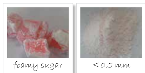
Figure 10: Homogenization of foamy sugar; left: original sample, right: sample ground to < 500 µm
