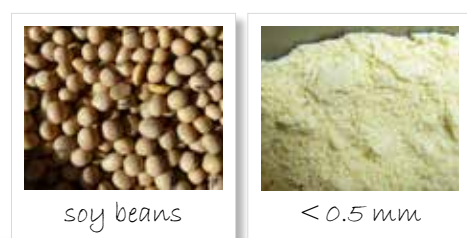
Figure 11: Homogenization of soy beans; left: original sample; right: sample ground to < 500 µm
