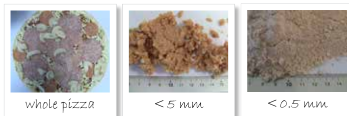
Figure 1: From left to right: a whole pizza; sample after grinding to coarse particles < 5 mm; fully homogenized sample with particle sizes < 0.5 mm
