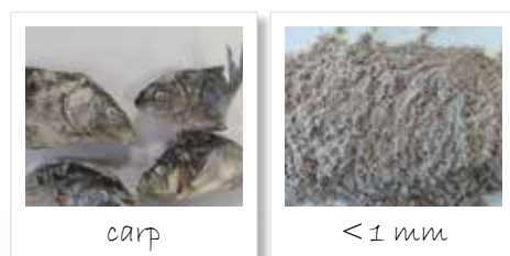
Figure 6: Homogenization of fish; left: original sample; right: sample ground to <1 mm
