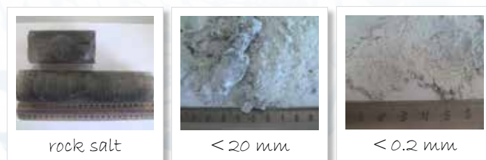
Figure 9: Homogenization of rock salt; left to right: original sample, sample ground to < 20\text{ mm} , sample ground to < 200\ \mu\text{m}
