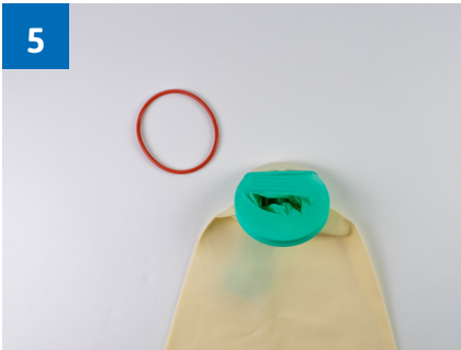
Pull the cuff of the glove over the connector
