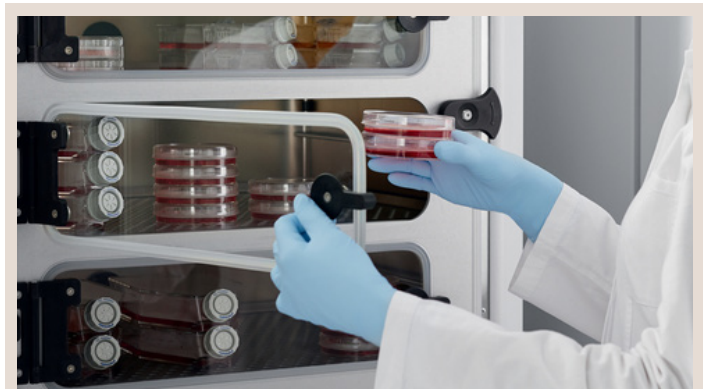
Figure 11: Split inner doors maintain the atmosphere inside the incubators.
